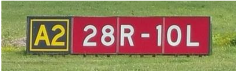
Figure A3.2. (NFARS) NFARS Information Sign (Taxiway Direction Sign with Location Sign).
