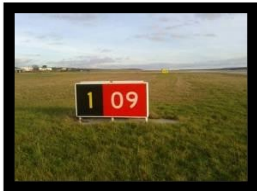
Figure 4.4. Intermediate Holding Position Signs.
