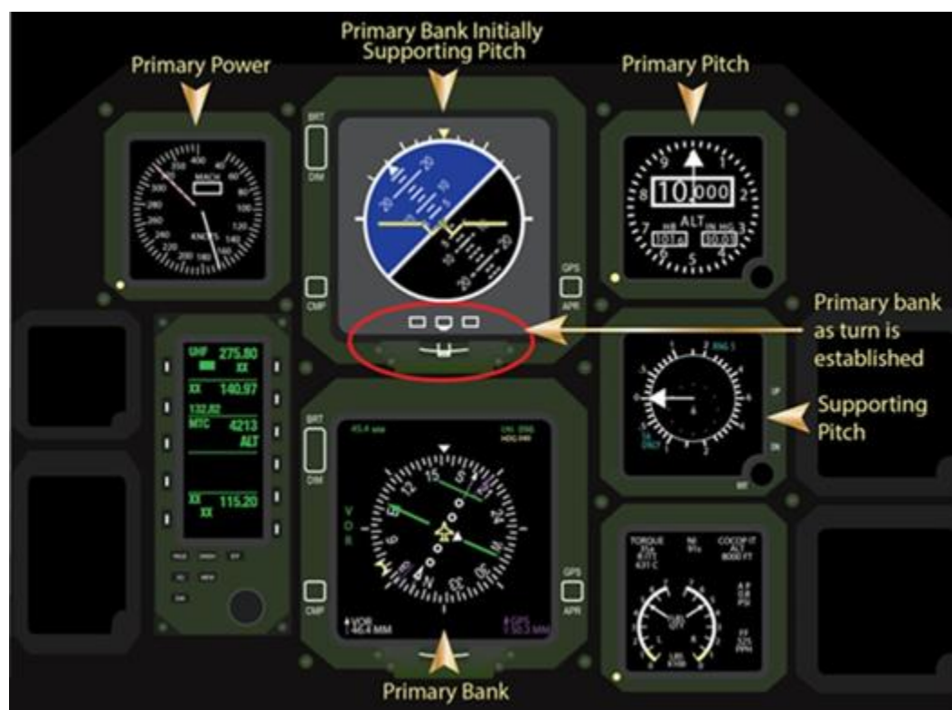
Figure A5.4. Level Turns.
