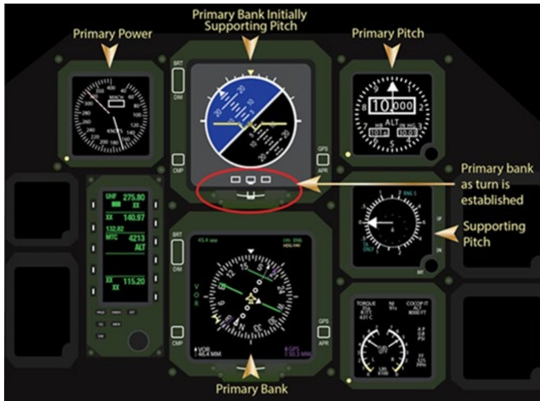
Figure A5.4. Level Turns.
