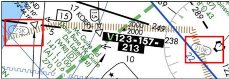
Figure 13.4. Maximum Holding Airspeed.
