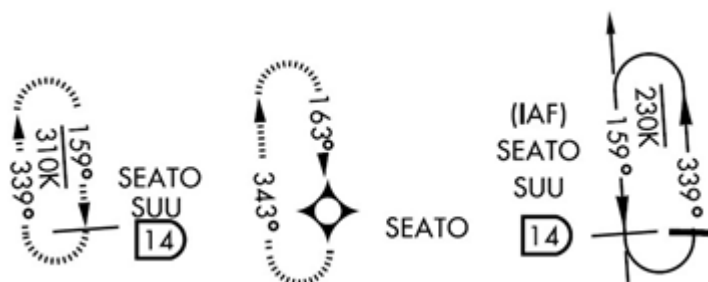
Figure 13.2. Multiple Holding Patterns at Same Fix.
