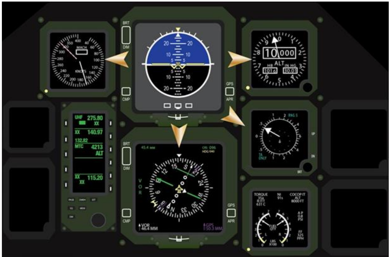
Figure A4.4. “Hub and Spoke” Cross-check.
