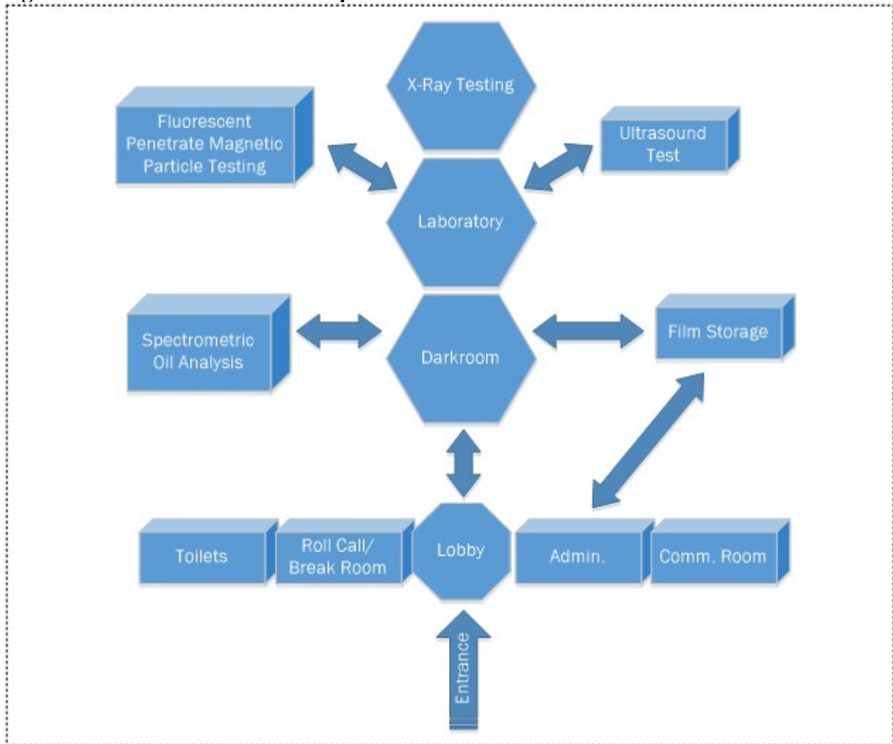
Figure 7.3.12. Non-Destructive Inspection Area.
